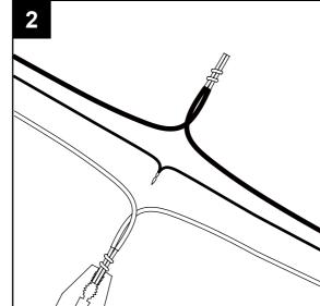
3. Attach wire nuts (BB). Tape wire nuts (BB) and wires together.
