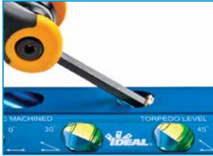
1. Remove the set screw with hex wrench
