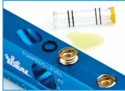
2. Remove O-ring and damaged vial
