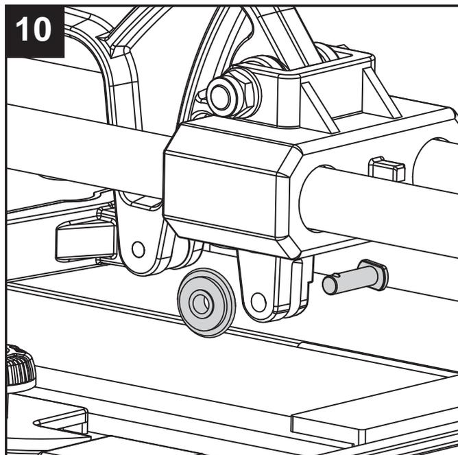
10. Remove the dulled cutting wheel.
