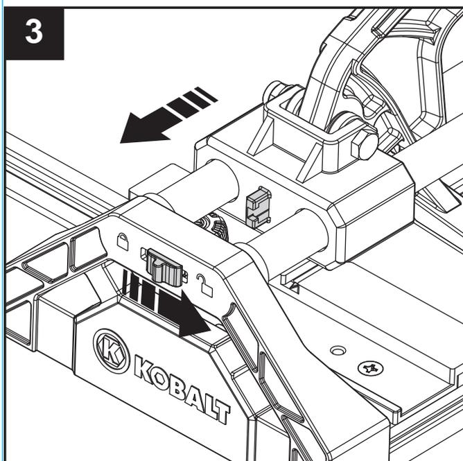
3. There is a lock on the front support (unlock it to release the grip handle before start using) which will hook the grip handle during movement of the tile cutter to avoid any sliding and impact.
