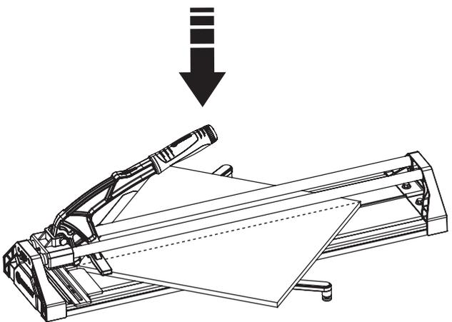
7. Align the breaker bar with tile corner, then press the grip handle.
