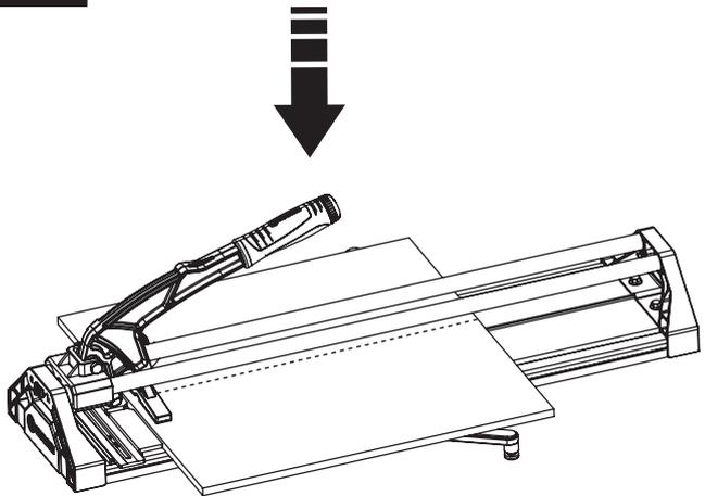
5. Align the breaker bar with tile front edge, then press the grip handle.
