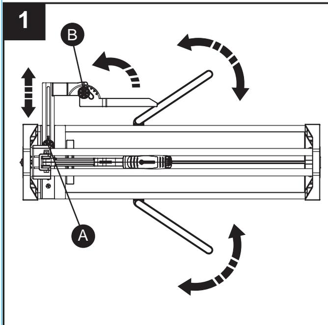
1. Position the extension arms, side rule (release knob A) and angle guide (release knob B) as desired to support stable positioning of tile (not included) for scoring.
