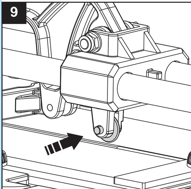
9. Push out the collar pin. The collar pin may require a strong push to be removed.
