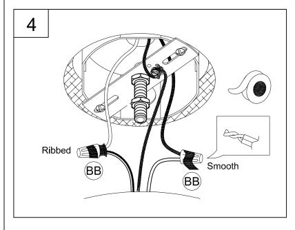
4. Strip 3/8" of insulation from the electrical wire ends. Using wire connectors (BB), connect the RIBBED fixture wire to the WHITE supply wire from the outlet box; connect the SMOOTH fixture wire to the BLACK supply wire from the outlet box.
