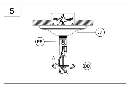
5. Tuck the wires into the outlet box and slip the canopy (JJ) over the chain holder (EE). Thread the screw collar (DD) onto the chain holder (EE) to secure the canopy (JJ) tightly to the ceiling.
