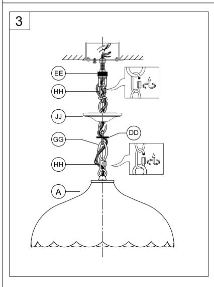
NOTE: During this step, determine the hanging length of your fixture by removing chain links (GG) and optionally cutting the electrical and ground wire to length.
