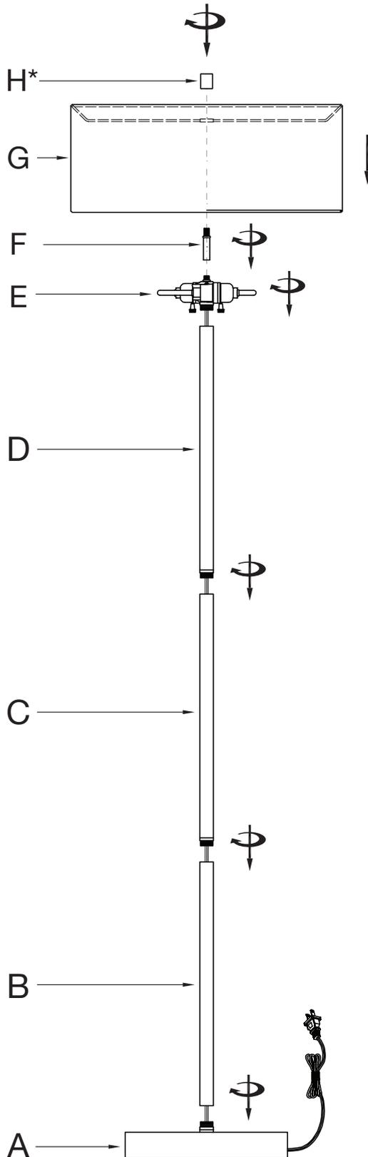
\* Part H (Finial) may come pre-installed to Part F (Shade Support). Unscrew Part H before installing Part G (Lampshade), then reinstall Part H to secure.
