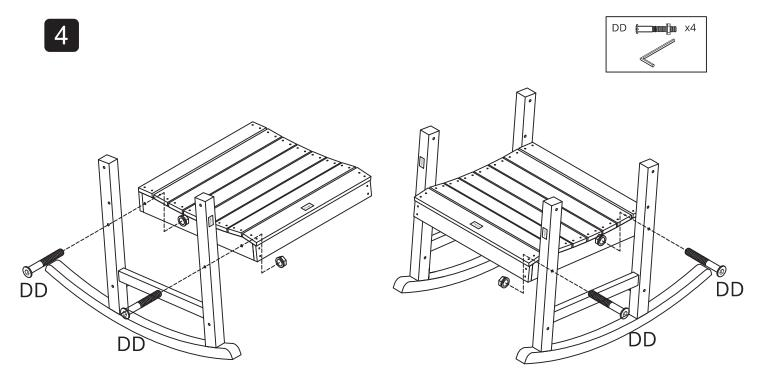
Do not fully tighten all bolts until Back A and Seat B are installed together.
