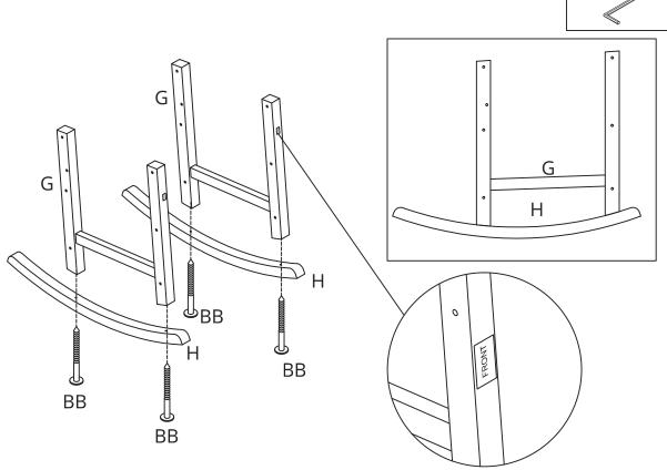
Notice: The front leg with 3 holes of the Frame(G) should be installed in the front position of the Rocker Bar(H).
