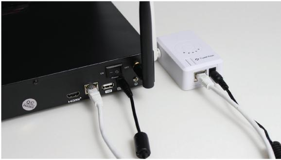
1. Have the Repeater next to the NVR system and plug in the power.
