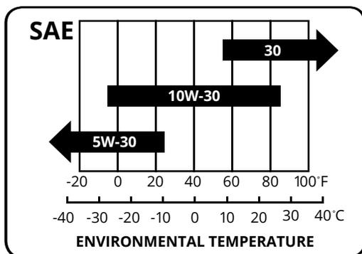
**Engine oil recommended: SAE 10W-30.** Viscosity varies with regions and temperatures. Choose your oil viscosity using the chart to the left.
