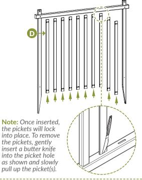
Slide a rail up the posts until the picket lock into the routed holes in the rail.
