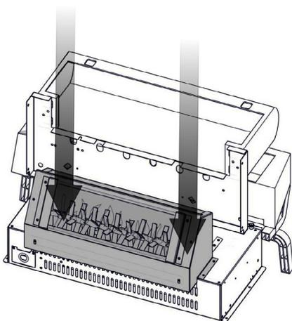
**INSTALL THE FLAME BOARD ASSEMBLY.
