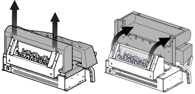
LIFT UP THE LOG MOUNTING PLATE, TURN IT 90 DEGREES AND PLACE IT ON THE FIREBOX.
