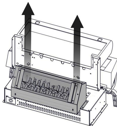
**REMOVE THE FLAME BOARD ASSEMBLY.
