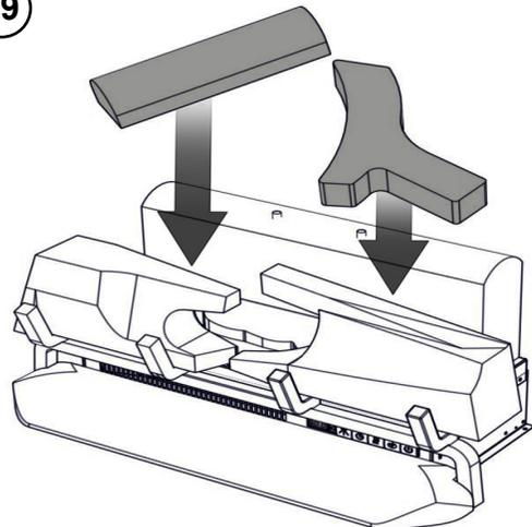
**PLACE REMAINING LOGS ON THE TOP AND REAR LOG.
