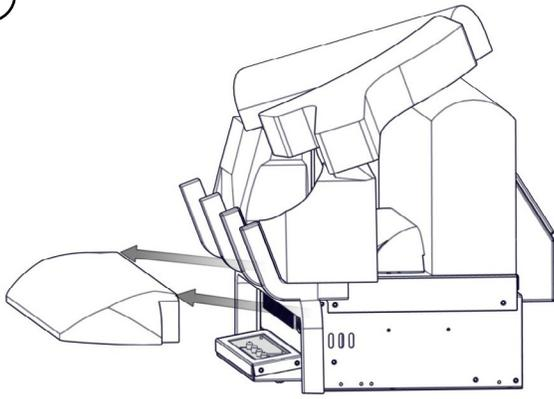
1. TO REPLACE FRONT EMBER BED (W135-0605) REMOVE THE DAMAGED EMBER BED AND REPLACE WITH NEW ONE.
