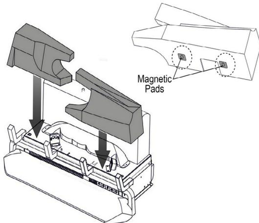
**PLACE FRONT TWO LOGS ON LOG MOUNTING PLATE.
