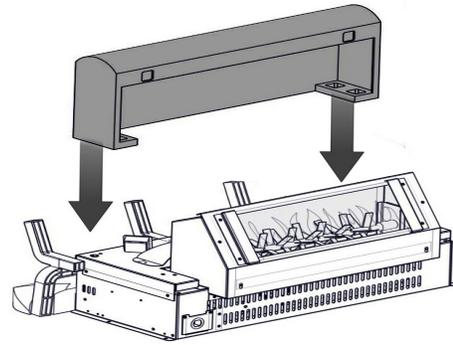
**PLACE THE REAR LOG ONTO LOG MOUNTING PLATE.
