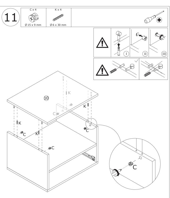
Cover plate 10 to the component with wooden dowel(K) and turn cam lock(C) clockwise to tighten as shown.
