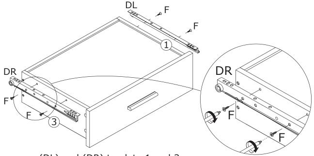
Fix runner(DL) and (DR) to plate 1 and 3 respectively with screw(F) as shown. Please pay attention to the holes where the accessories are inserted.  $_{8/16}$
