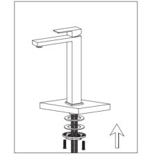
3. Re-install the rubber washer followed by the metal washer and lock nut,then hand tighten it.
