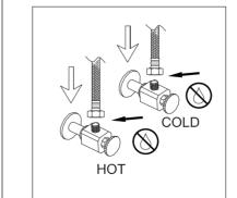
Connect hoses to the water supply and tighten.Check all connections at arrows for leaks.Retighten if necessary,but do not overtighten.
