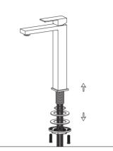
1. Remove the rubber washer,metal washer and lock nut from the faucet.
