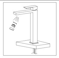
Remove the aerator and turn on faucet for 1-minute to flush debris from faucet and feed lines.Turn faucet off and re-install aerator.
