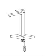
4. Hand tighten further using a screw driver to tighten lock nut screws.
