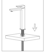
2. Install faucet with oring under the flange through center hole.
