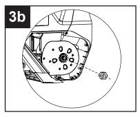
Remove the nut from the right of the axle.
