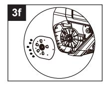
Remove the 6 screws that secure the left side plate.
