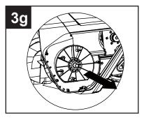
Pull the axle and remove the old impeller. Install the new impeller and insert the axle.
