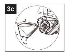
Remove the 5 screws that secure the left side cover.
