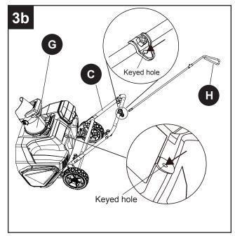
3c. Rotate the handle (H) on the chute control rod to ensure that it moves in the opposite direction as the chute.
