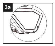
Remove the 5 screws that secure the right side cover.
