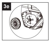
Using a socket (not included), remove the the large pulley inside the left side cover.
