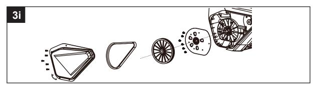
Reinstall the left side plate, large pulley, belt and left side cover.
