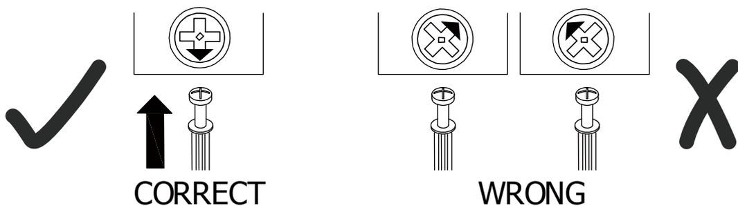
Nut should be in the centred of the cam lock when the two panels are joined.
