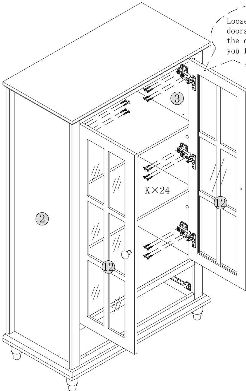
Loose the screw to adjust the doors to make them aligned, if the doors are not aligned when you finish the assembly.
