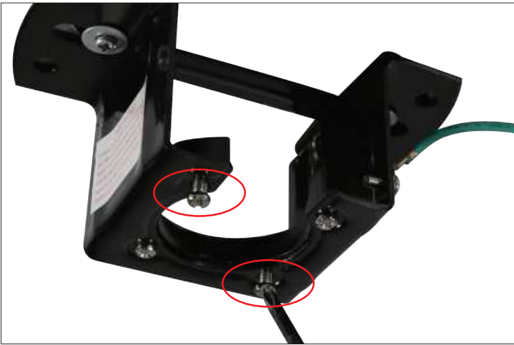
Step 2 Loosen the two opposite screws
