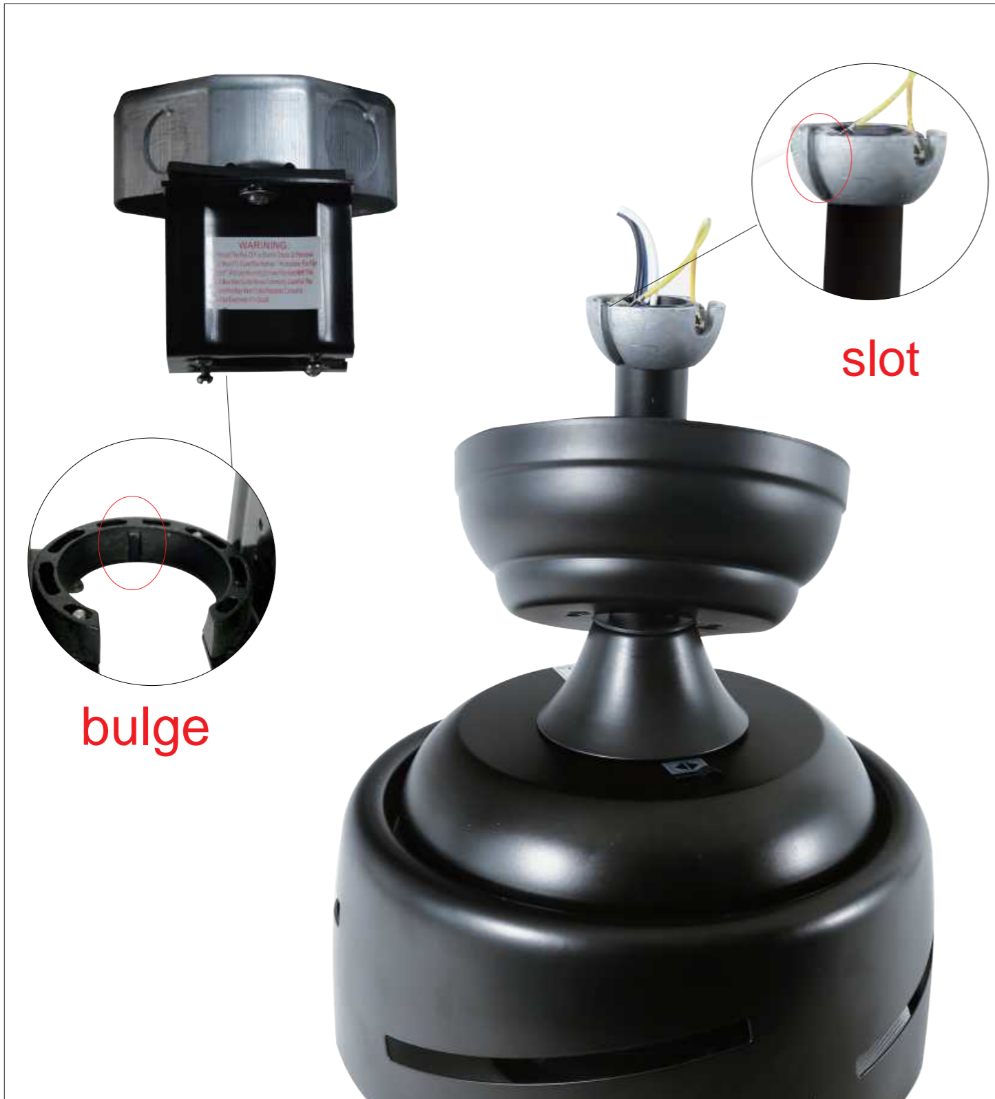
Step 10 Hang the fan on the hanging bracket and align the slot on the downrod with the bulge on the hanging bracket.
