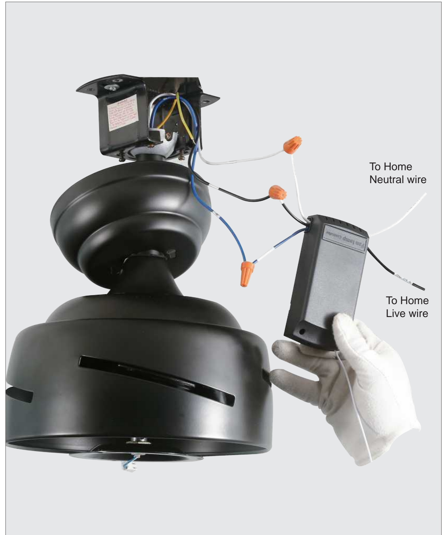
Step 11 Connect the wires from the motor to those three wires on one side of the receiver. Black to Black, White to White, Blue to Blue
