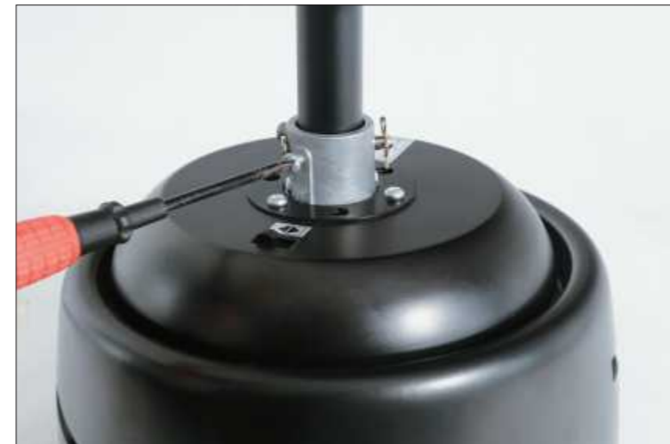
Step 8 ① Tighten the two screws on the coupler. ② Insert the Cross pin and R-pin.
