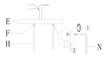
5 » If needed, shorten the extra length of the fixture wires from cords (H) so that they all are at least 6 inches (152.4 mm) long above canopy (E) within the outlet box.
