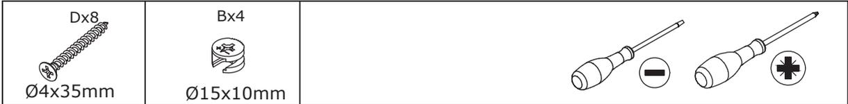
Insert cam locks(B) into board 9 and 11 as shown, turn cam locks clockwise to tighten. Slide board 12 into available slots. Attach board 10 to the component with screw(D) as shown.
