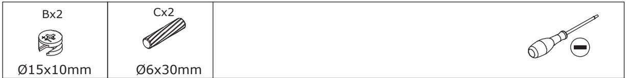
Connect board 7 to 4 with wooden dowel(C) and turn cam lock(B) clockwise to tighten as shown.
