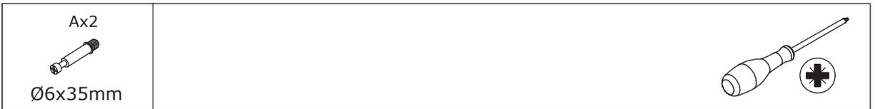
Insert quickfit screw(A) into corresponding holes in board 6 with a screwdriver as shown.
