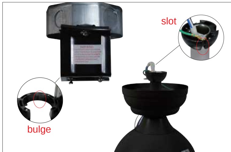
Step 9 Hang the fan on the hanging bracket and align the slot on the downrod with the bulge on the hanging bracket.
