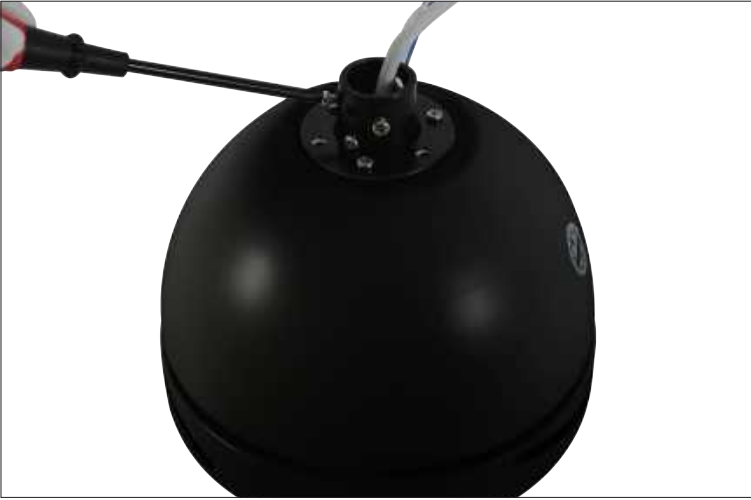
Step 3 Loosen the 2 screws on the coupler.
