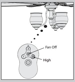
**Note:** The remote must be paired before the fan will operate.
