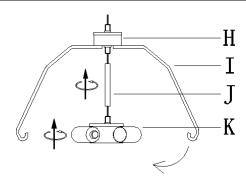
4. Pass the fixture wires through stem (G) and canopy (E), then screw them onto arms assembly (H).
