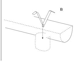
Hook Rain Chain (B) onto Gutter Clip (A). Wait for rain and enjoy! STEP 3 Note: Use a filter screen to prevent leaves and debris from dropping into your rain chain if needed.
