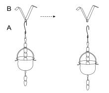
**STEP 2** Slide the Gutter Clip (B) into the rain gutter drain hole.
