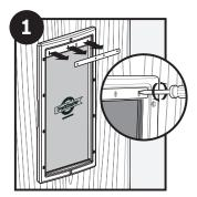
**To Replace** vinyl flap, remove flap screws and flap support from top of pet door frame.
