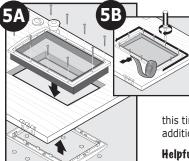
**5A** Place interior frame (frame with 2 flaps) into cut-out. Next place exterior frame into cut-out from under side of door, inserting core covers inside tabs of frame. Hold frame together. Insert nylon screws through holes in interior frame into holes in exterior frame. Thread a bex put onto bottom of each screw.
