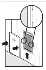
The Closing Panel snaps onto the interior frame of the Extreme Weather Pet Door™. It is useful during inclement weather or to keep your pet from using the pet door.
