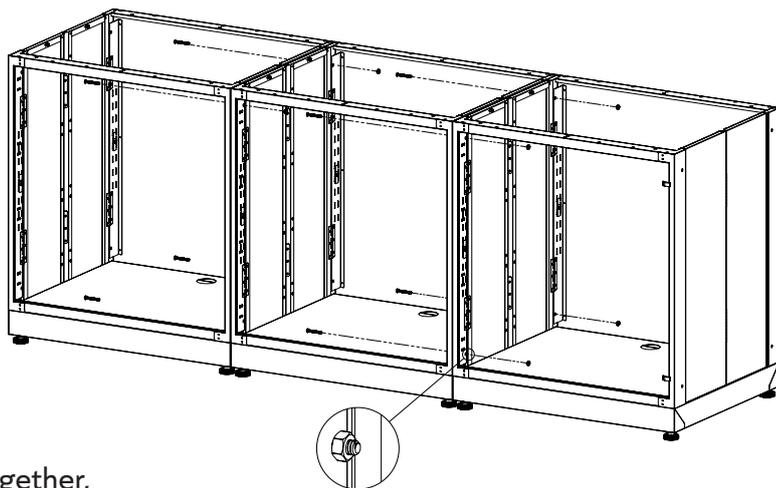
Once your double or triple cabinets are bolted together, install 2 top brackets (J) for your Double cabinet set up and 4 top brackets (J) for your triple cabinet setup. Bolt the top bracket (J) to the top of each interior side panel with 2 bolts (I) per bracket as shown. J
