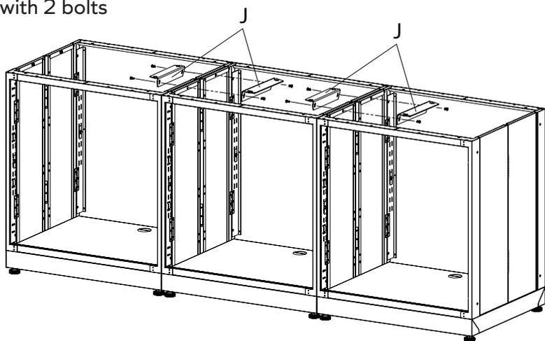
With four or six people, for the triple wide tops, lift your Stainless Steel top in place over the cabinets body with the arrow sticker pointing to the back of the cabinet. The flanges on the bottom sides of the top should slide into place inside the edges of the cabinet. You may need one person to push the center of the sides of the cabinet out (the hinge may have folded in a little) to make sure the flanges are all inside the body of the cabinet.
