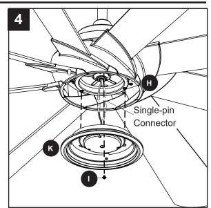
5. Lift the glass bowl (L) over the light kit (K) and turn in a clockwise direction until it is secure.
