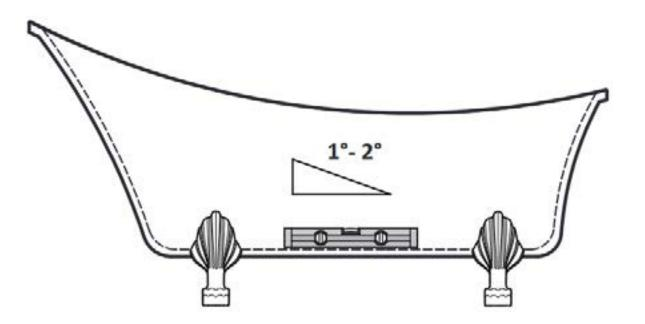
20. Place a level inside the tub. Make sure the bathtub is stable and that all legs rest perfectly on the floor, if not, ad-just the levelling pads.
