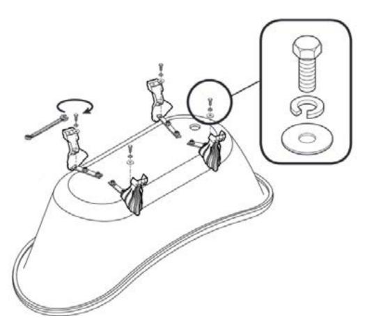
4. Hand tighten the nut so the bar can still slide back and forth in case you have to center it after the feet are installed.
