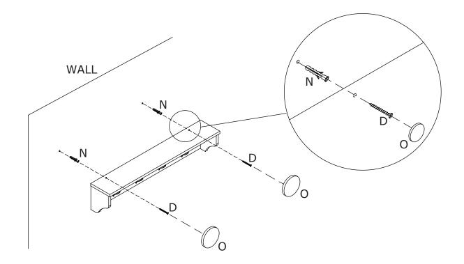
Drill holes on your wall, knock into part(N). Fix the component(assembled in step 3) to wall using screw(D) as shown. Use sticker(O) to cover screw(D).
