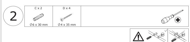
Connect plate 2 and 3 with plate 4 using wooden dowel(C) and fix using screw(D) as shown
