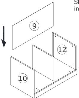
Slide plate 9 along grooves in plate 10 and 12.
