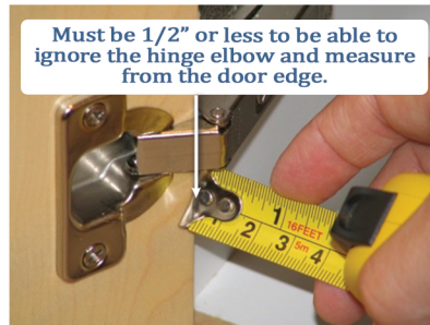
You can take advantage of the space created under the protruding hinges as long as the elbow doesn't protrude into the opening more than 1/2 inch.
