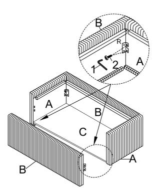
Align other long panel (#B) and attach with bolts (#2)
