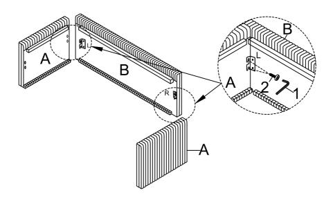
Align both short panels (#A) against a long panel (#B). Secure connectors (#4) with bolts (#2)
