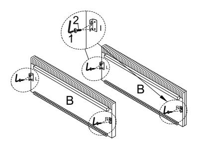
Attach connectors (#4) to each side of the long panels (#B) with bolts (#2) and Allen wrench (#1)
