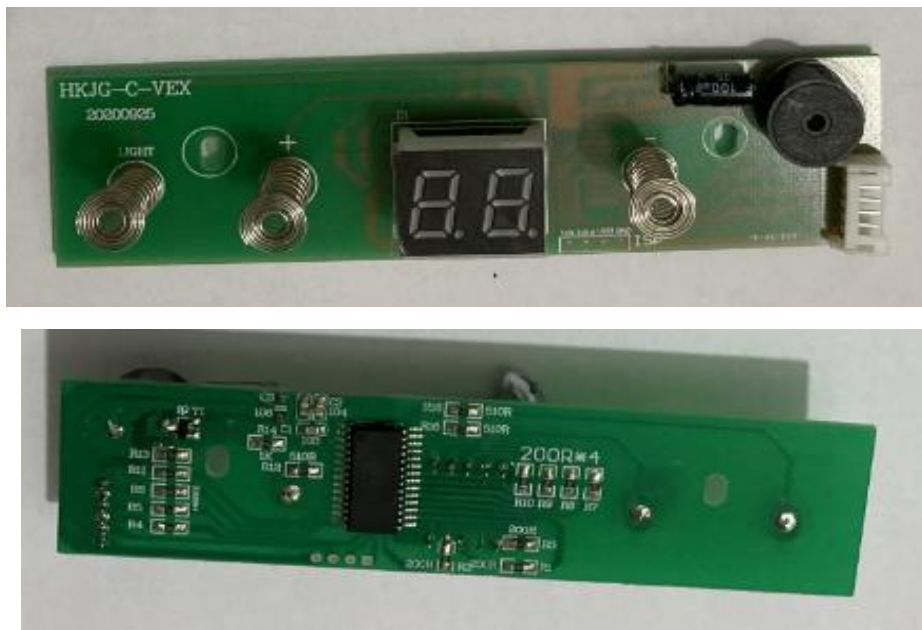
Photo 48 - Alternative electronic controller of models JC-75VEX-F
