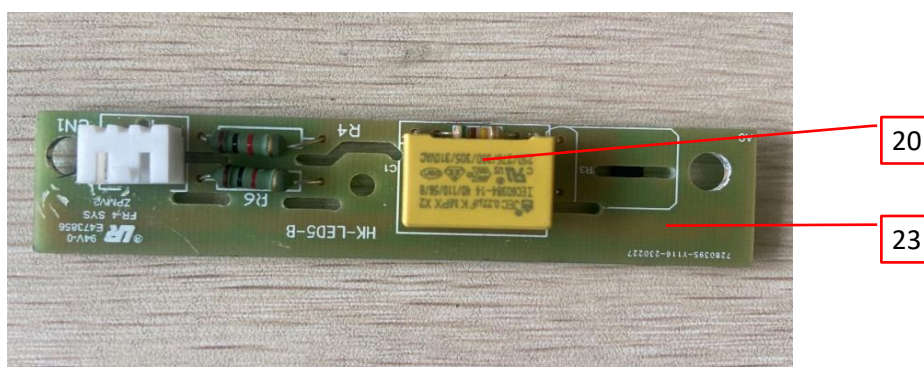
Photo 27d - Alternative PWB for LED lamp
