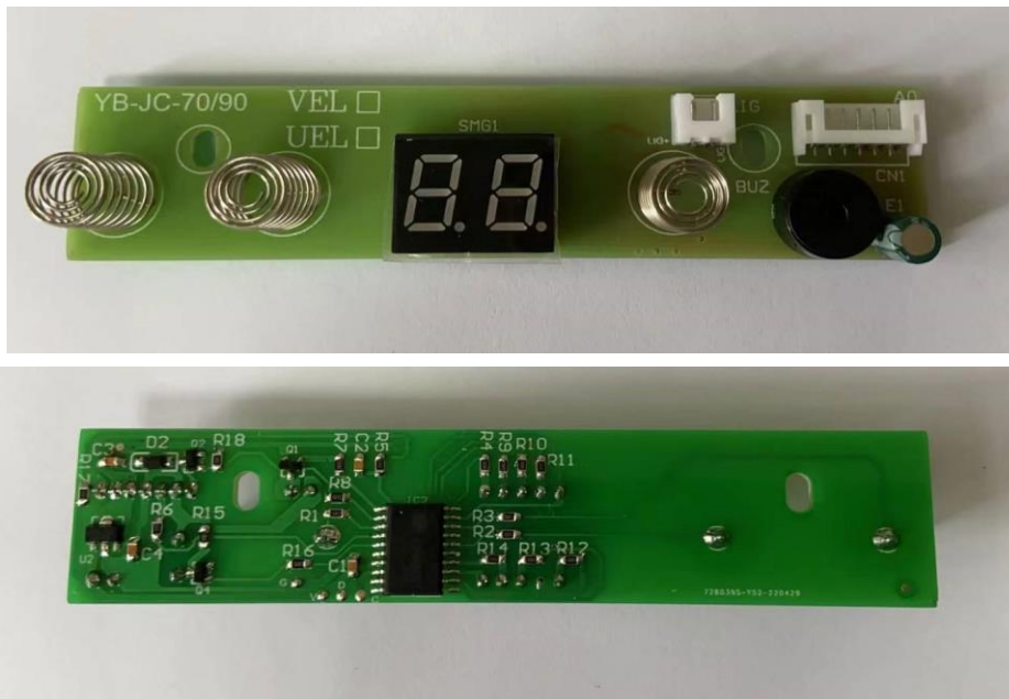
Photo 62 - Alternative control panel PWB of models JC-*UEL-F, JC-*VEL-F (*=36, 46, 48, 70, 75, 90)
