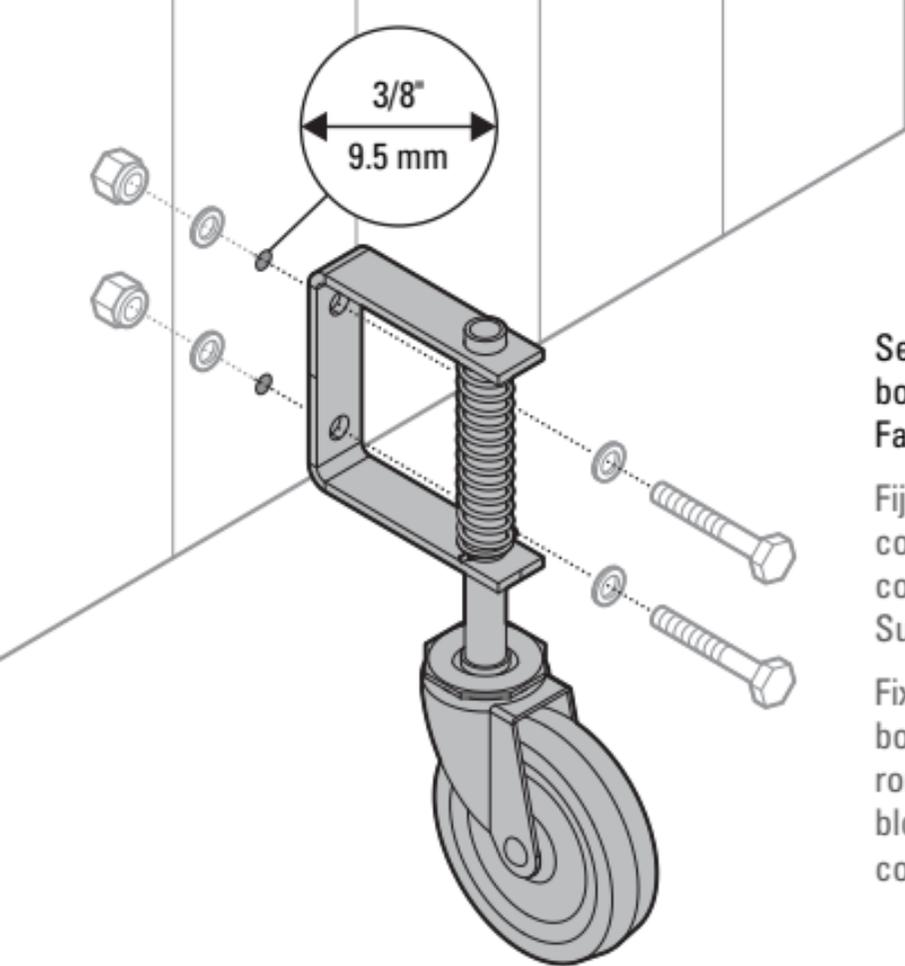
Secure castor to gate with 5/16" bolts, washers, and lock nuts. Fasteners not included.
