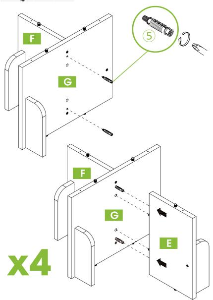
As shown in the figure, connect and fix the parts C, E, F and G respectively with 8 self-tapping screws ②
