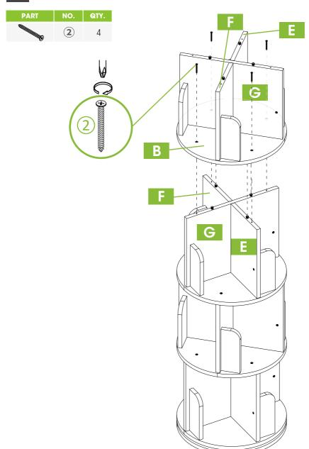
As shown in the figure, connect and fix Parts A, E, F and G with 4 self-tapping screws 2
