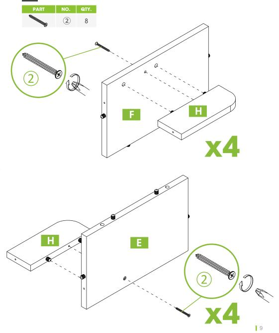
As shown in the figure, connect Parts G and H, G and F respectively with 16 self-tapping screws 2
