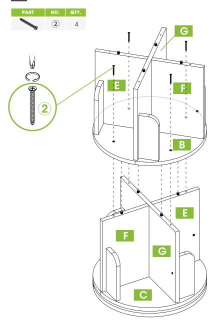
As shown in the figure, connect and fix Parts B, E, F and G with 4 self-tapping screws ②
