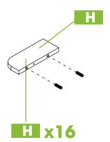
As shown in the figure, connect Parts F and H, E and H respectively with 8 self-tapping screws ②
