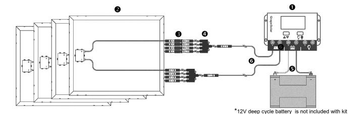
Remove the panel covering. In good sunlight, the charge controller's • "BAT %" should increase to 100%. When the controller is set to "LOAD ON," the system will provide power through the load control output or through the USB port.
