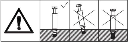
Insert quickfit screw(A) into plate 2 and 3 with a screwdriver as shown.
