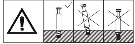
Fix part(E) to plate 1 with screw(O) as shown.
