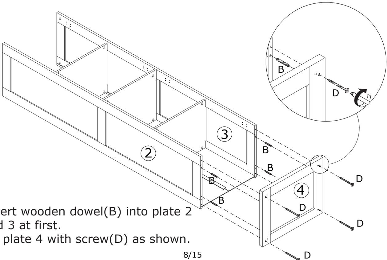
Insert wooden dowel(B) into plate 2 and 3 at first.
