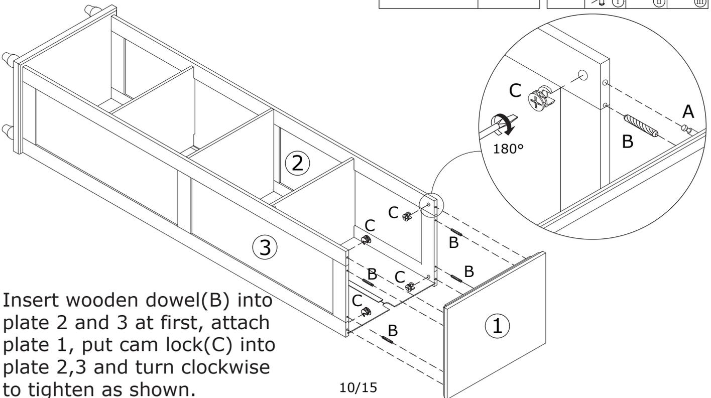
Insert wooden dowel(B) into plate 2 and 3 at first, attach plate 1, put cam lock(C) into plate 2,3 and turn clockwise to tighten as shown.
