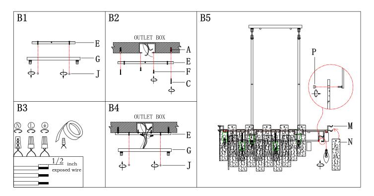
Step B1 » Unscrew knob nuts (J) and carefully remove mounting plate assembly (E).
