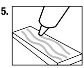
Use "Liquid Nail" or "PL Adhesive". Apply a generous amount to the back of the splash.
