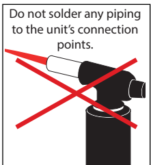
Figure 5 - DO NOT SOLDER TO THE UNIT
