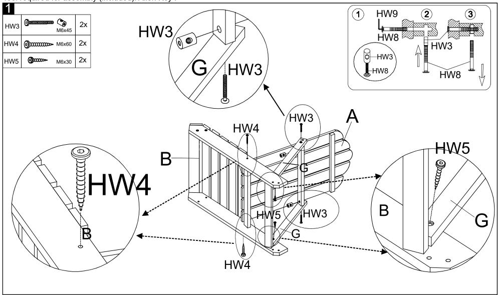
Step 1: Attach the Back (A) ,support back (G) to the Seat (B) as shown in the picture .Using the Screw L (HW4), T Bolt & nut (HW3) to tighten both side by the Allen key (HW9) and Extra bolt (HW8). After that using the Screw S (HW5) to fix the Support back (G) to the Seat (B) both side by using the Allen key (HW9) as shown on the picture.
