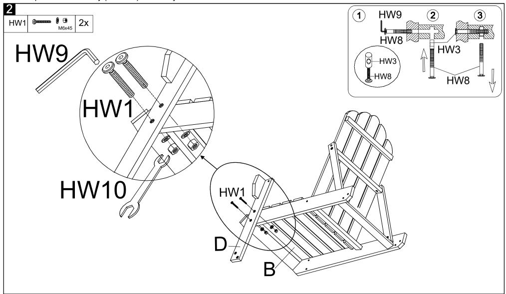
Step 2: Attach the Left leg (D) to the Seat (B) as shown on the picture. Using the Bolts and nut (HW1) and tighten with the Allen key (HW9) and Wrench (HW10).
