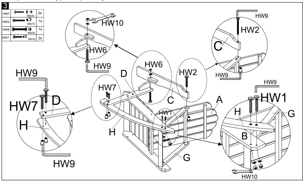
Step 3: Attach the Left Arm (C) to the Left leg (D) as shown on the picture. Using the Bolt and round nut L ( HW2) fix the Left arm (C) to the Support (G), then using the Bolt & nut (HW6) tighten to the Leg (D) by the Allen key (HW9) and Wrench (HW10) as shown on the picture. Attach the Left base leg (H) to the chair ,using the Bolt & round nut S (HW7) in the front, the Bolt and nut (HW1) in the back. Tighten it by the Allen key (HW9) and Wrench (HW10) as shown on the pictures.
