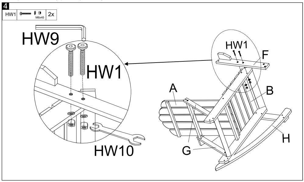
Step 4: attach the Right leg (F) to the Seat (B) as shown on the picture. Using the Bolt and nut (HW1) to tighten by using the Allen key (HW9) and Wrench (HW10) as shown on the picture.
