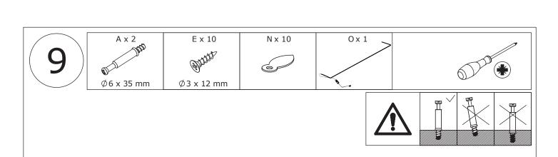
Screw eccentric rod(A) into panel 13 at first.
