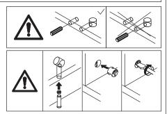
Attach panel 13 to panel 12 using wooden dowel(C), add cam lock(B) into panel 12 and turn clockwise to tighten as shown.
