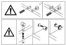
Attach the component(assembled in step 17) to panel 13, 14, 15, 16, 17 and 19 using wooden dowel(C), add cam lock(B) into and turn clockwise to tighten as shown.
