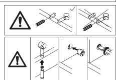
Attach panel 6 and 7 to panel 3 using wooden dowel(C), add cam lock(B) into panel 6,7 and turn clockwise to tighten as shown.
