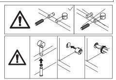
Attach the component(assembled in step 13) to panel 13, 18 and 14 using wooden dowel(C), add cam lock(B) into and turn clockwise to tighten as shown.
