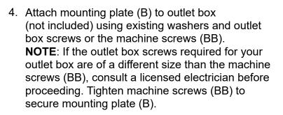
**CAUTION:** The fixture must be mounted to an outlet box that is supported by the building structure. Plastic outlet boxes are not recommended.
