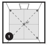
After thoroughly cleaning the subfloor, measure the space to determine the center point of the room. Strike a line at this point. Create a 90° angle to divide the room into four equal parts.
