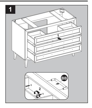
As shown in the diagram, fully extend the drawer and locate the plastic levers on the metal glide tracks. Push the left-side and right-side levers at the same time to disengage the drawer from the drawer glides. Gently lift the drawer up to remove it from vanity (A).
