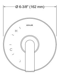
2-3/4" (70 mm) Thin Wall 3-1/2" (89 mm) Thick Wall If over 3-1/2" (89 mm) and up to 4-1/4" (108 mm), use Deep Roughing-in Kit
