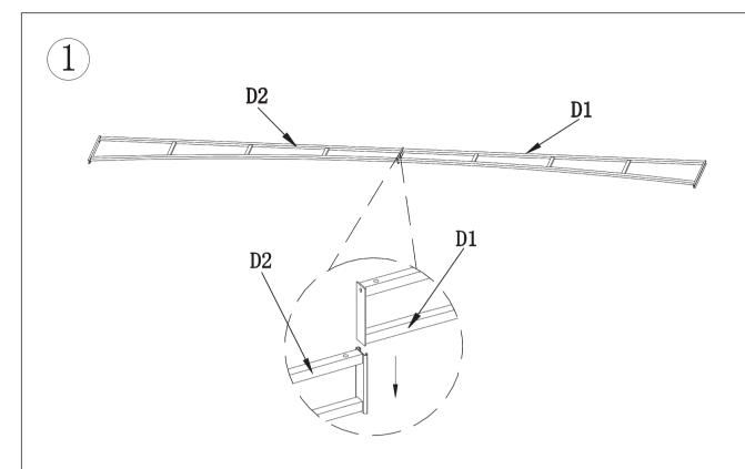
Connect two Long Side Beams(D1) to Long Side Beams(D2).
