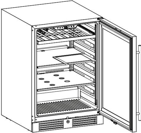
1. Open the door completely unload any content within the beverage cooler. Make sure the shelf is pushed back completely.
