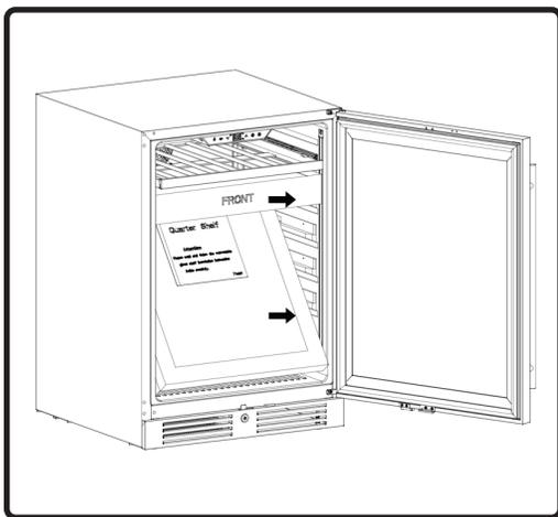
1. Remove foam from the regular glass shelf. Remove the box containing the retractable glass quarter shelf.
