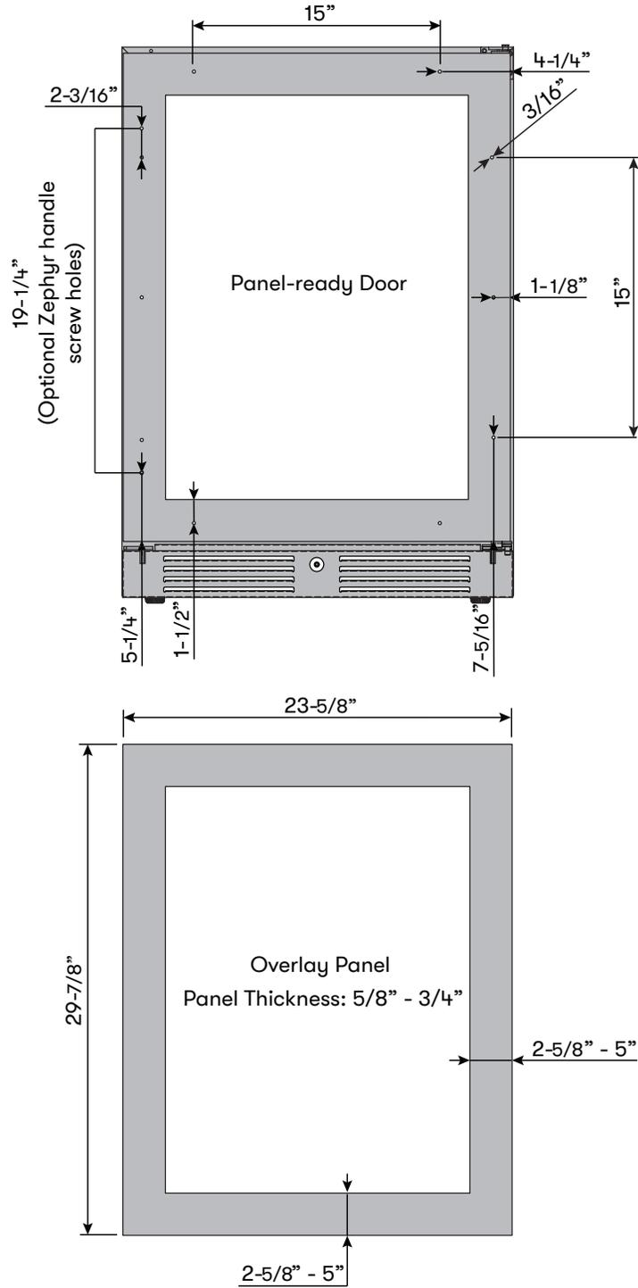
**NOTE:** Compatible with framed overlay panels only. The weight limit for the overlay panel is 22 pounds.
