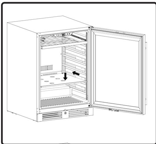
3. Relocate the regular glass shelf to one of the bottom two ledges. Make sure the shelf is completely pushed back.
