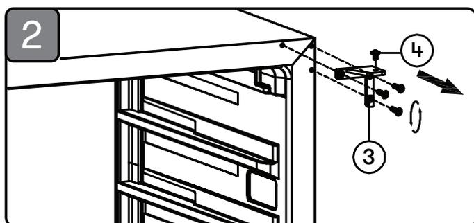
2. Remove the 3 hinge screws from the top right hinge (3) and remove the top right hinge.
