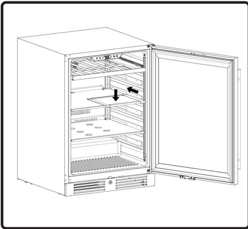
5. Carefully install the retractable glass quarter shelf in the desired position.
