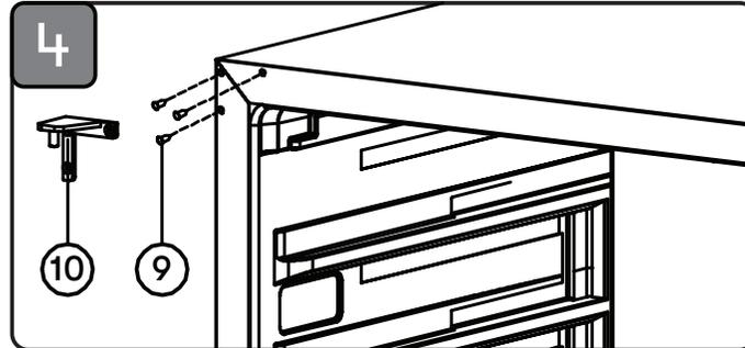
4. Remove the 3 black decorative nails (9) from the top left of the cabinet. Install the black decorative covers to the top right of the cabinet and install the new top hinge (10) from the hardware package that includes the installation manual at the top left of the cabinet with 3 screws.
