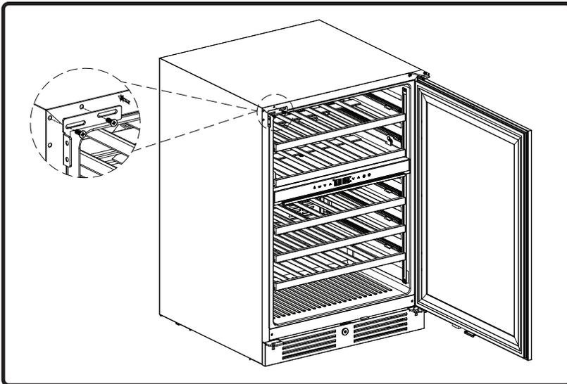
1. Open the door and pry off the black decorative nails. Place the anti-tip bracket on the cooler and secure with (2) M4\*12 flathead screws.
