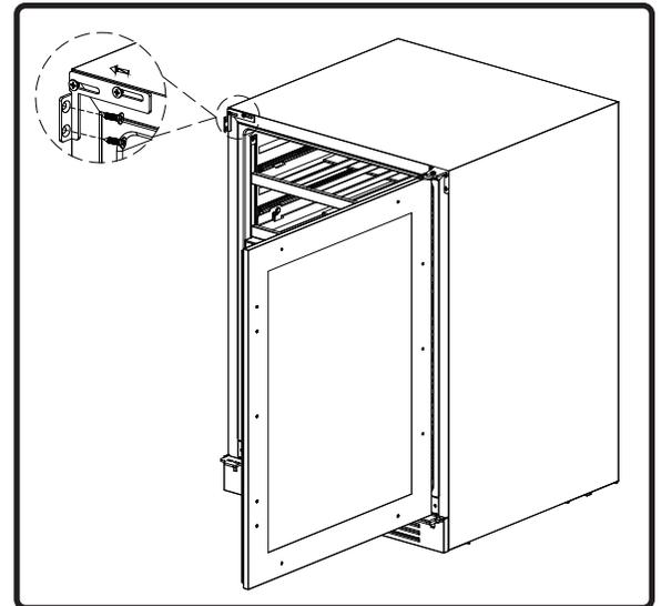
2. Push the cooler into the desired location for installation. Open the door and install the anti-tip bracket onto the cabinet with (2) ST4\*12 self-tapping screws.
