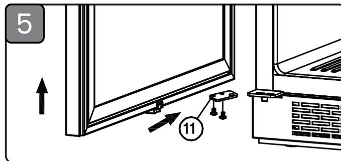
5. Install the lower door axis (11) and install the door once correctly aligned. Secure the door with the top screw on top of the hinge (4).
