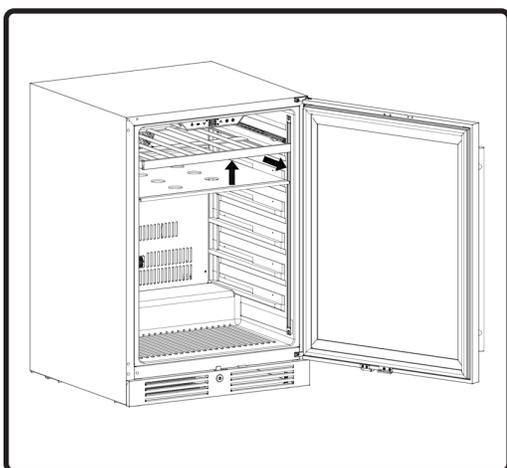
2. Lift either the left or right side of the shelf to create a 45° angle from its original position and pull the shelf outward.
