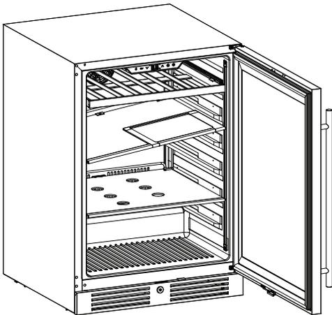
2. Lift either the left or right side of the shelf to create a 45° angle from its original position. Make sure not to lift either side of the shelf too hard as it may come in contact with the inner wall mount.
