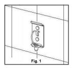
Place the Quick-Mount design mounting plate(s), Fig. 1, vertically at the corresponding location(s) on wall with the spring-pin on the bottom side. Then, mark the screw holes locations on wall through the upper & lower holes at mounting plate.
