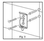
3) Push plastic anchors provided into the holes until flush with wall. Then, screw mounting plate to the wall with the screws provided, with spring-pin on bottom side, Fig. 3.
