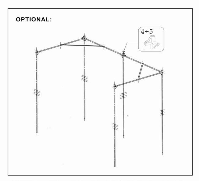
OPTIONAL: To add a second adjacent Veggie Wal® I Kit to the same garden bed, attach one L-connector(4) to a T-connector (5) as shown in the diagram attached. When you do this, one vertical tube is not needed.
