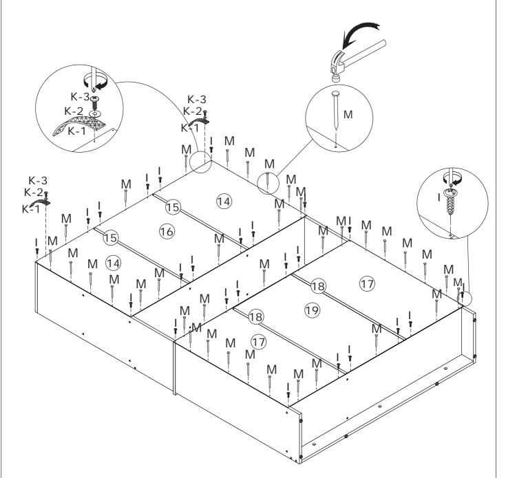
Fix part(K-1) to back plate with washer(K-2) and screw (K-3) as shown.
