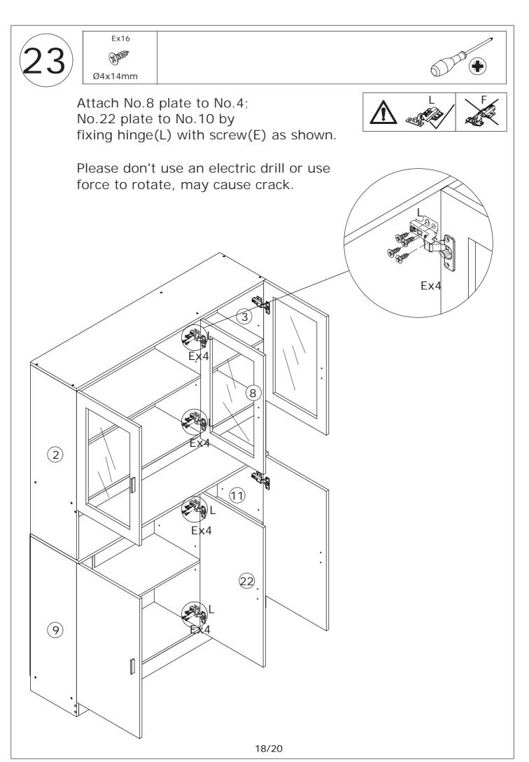
If there is misalignment after you install, adjust the screw to the best condition.
