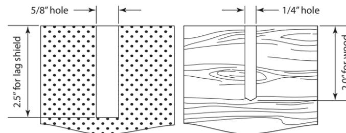
**5 For hardscape:** Remove any debris from the hole and insert the lag shield so it is flush with the surface. Screw the mounting bolt into the lag shield.
