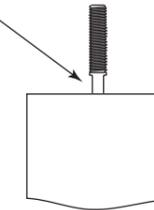
**6** Carefully screw the four leveling feet into the bottom of each leg about half way.
