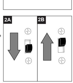
2C. **IMPORTANT**: Reverse switch must be set either *completely UP* or *completely DOWN* for fan to function. If the reverse switch is set in the *middle* position, fan will not operate.
