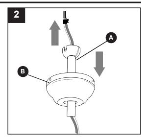
Slip downrod (A) into yoke, align holes and re-install pin (K) and clip (L). Tighten set screws in yoke and then tighten nuts on the set screws.
