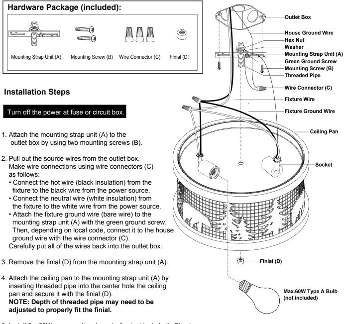
6. Install 2 x 60W max. medium base bulbs (not included). Check relamping label at socket area or packaging for maximum wattage allowed.
